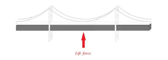
Main goal: Computing an explicit threshold for the appearance of lift on the deck of a bridge. Engineers evaluate the lift force exploiting wind tunnel tests:
