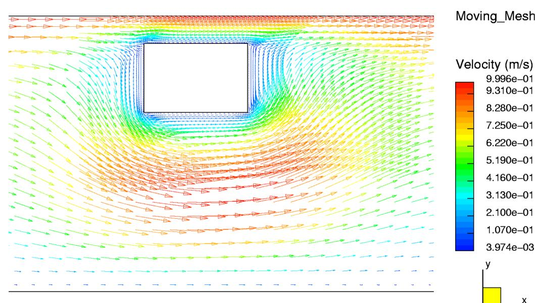
Field of relative velocity in body vicinity, obtained by subtracting body velocity from the absolute velocity field computed using a moving mesh: almost identical to the result obtained in the moving reference frame...
