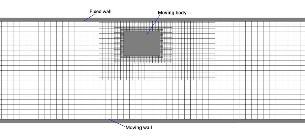
Test case for flow around a body moving in a channel with constant velocity (from right to left): the mesh is locally refined around the body. The flow is laminar (Reynolds number of the order of 1). The solution domain is larger than the figure shows.
