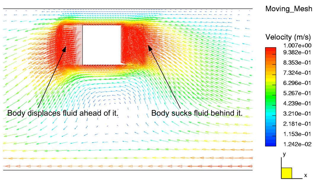
• Field of absolute velocity in body vicinity, computed using a moving mesh.
