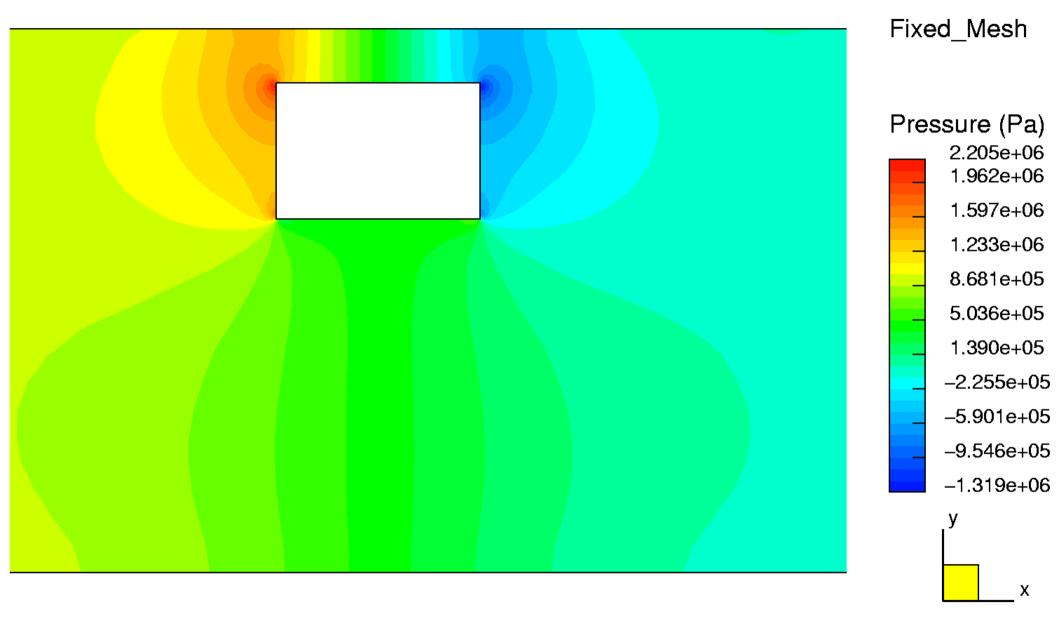
Pressure field in body vicinity, obtained from a steady analysis in a bodyfixed coordinate system.
