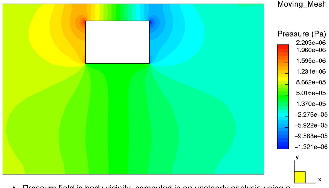
Pressure field in body vicinity, computed in an unsteady analysis using a moving mesh – almost identical to the solution obtained using MRF...
