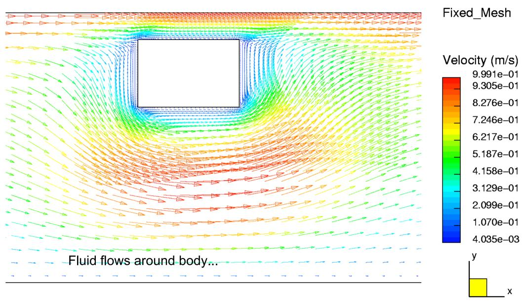
• Field of relative velocity in body vicinity, computed using a fixed mesh and a coordinate system moving with the body.
